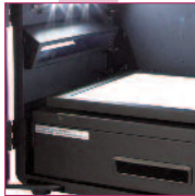
White light table – use plug-in white light table to view coomassie blue and silver stain protein gels; may also be used to view tissue slides and autoradiographs
